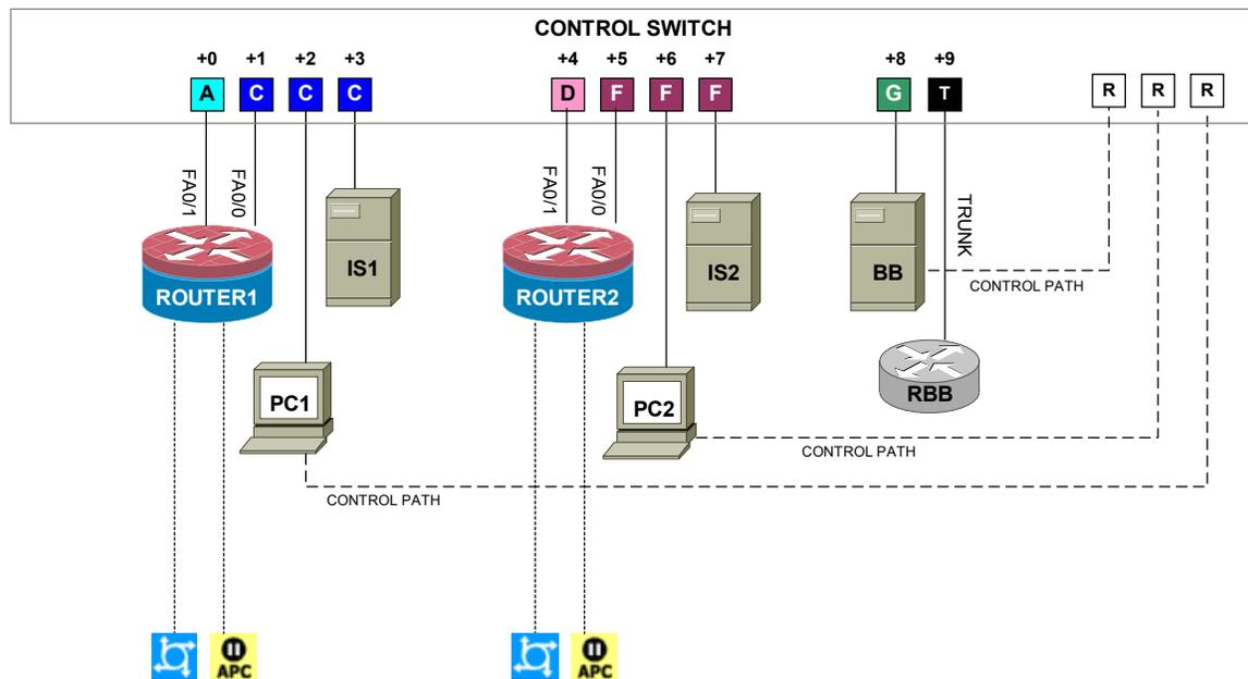
⇒ The actual FNS labs refer to SW0. This device is not implemented in NETLAB<sub>AE</sub>. In addition, the NETLAB<sub>AE</sub> cable scheme (depicted above) is different from SW0.
