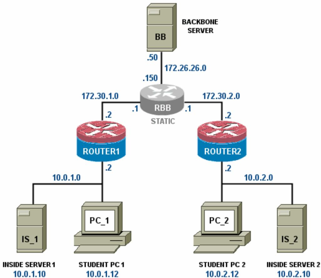
You may have up to two Security Router Pods per NETLAB<sub>AE</sub> system.
