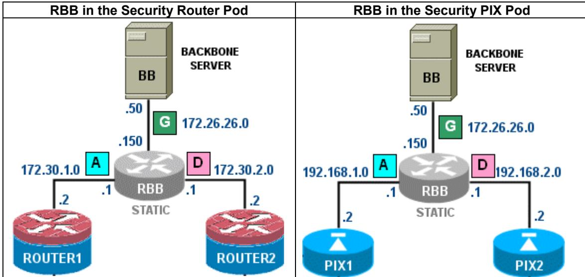
Similar to section 8.2, we determine that the BASE VLAN for POD\_5 and POD\_6 is 140 and 150 respectively. We compute the VLANs for network A, D, and G by adding the base VLAN for each pod to the offsets shown below.
