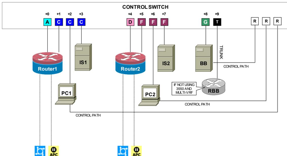
In the Security Router Pod, RBB performs routing between network **A**, **D**, and **G**. RBB advertises routes to its peers using both EIGRP and RIP version 2. EIGRP is used in most of the FNSR labs. RIPv2 is used in the Route Authentication and Filtering lab.
