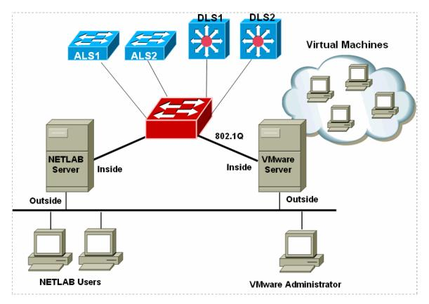
Once you have allocated a reserved port on the control switch, connect the VMware Server inside NIC using a straight through CAT5 cable. Configure the switch port as a trunk and allow only the VLANs that were bound to the VMnets. If your VMware server hosts virtual machines for more than one pod, allow all the relevant VLANs for each pod.
