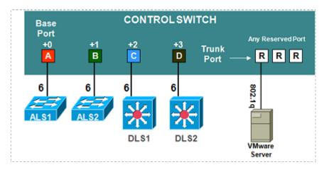
Ports are labeled +0 to +3 in the diagram and are relative to the *base port*. These ports must be consecutive on the same control switch. As with all pods, you choose a base port for the pod during pod installation (section 5). A control switch can support multiple pods. To determine the actual port numbers used for this pod, add the base port number to the relative port numbers shown in the diagram. For example, if the base port is 5, the actual port numbers will be 5 to 8.
