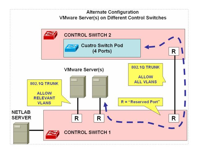
Ports connecting to VMware servers should only allow the VLANs associated with the pods being served. In addition, "switchport nonegotiate" should be used to suppress Dynamic Trunk Protocol (DTP):
