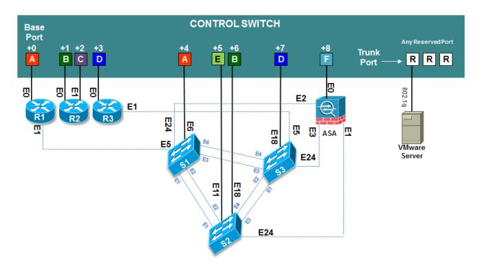
Ports are labeled **+0** to **+8** in the diagram and are relative to the *base port*. These ports must be consecutive on the same control switch. As with all pods, you choose a base port for the pod during pod installation. A control switch can support multiple pods. To determine the actual port numbers used for this pod, add the base port number to the relative port numbers shown in the diagram. For example, if the base port is 5, the actual port numbers will be 5 to 13.
