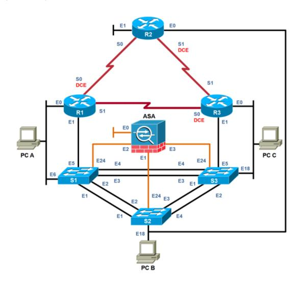
The *Multi-Purpose Academy Pod with ASA (MAP w/ASA)* features direct access to router, switch, and ASA consoles. Integration with a separate *VMware* server supports up to 3 virtual PCs. *NETLAB+* can provide remote access to the keyboard, video, and mouse of the *VMware* virtual machines in the pod.
