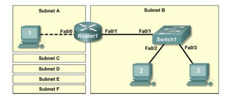
This topology requires two (2) FastEthernet interfaces. Physical router R2 in the NFP topology is used for the router activities in the diagram above, and therefore must have two FastEthernet interfaces. See section 2.1 for specific equipment requirements.
