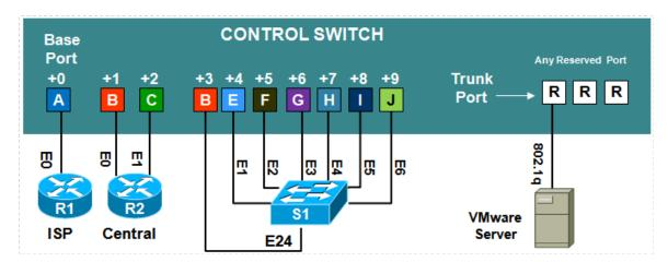
Ports are labeled +0 to +9 in the diagram and are relative to the *base port*. These ports must be consecutive on the same control switch.
