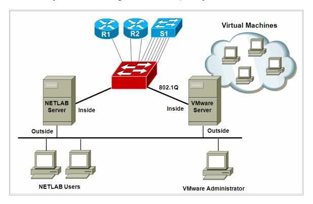
Once you have allocated a reserved port on the control switch, connect the VMware Server inside NIC using a straight through CAT5 cable. Configure the switch port as a trunk and allow only the VLANs that were bound to the VMnets. If your VMware server hosts virtual machines for more than one pod, allow all the relevant VLANs for each pod.
