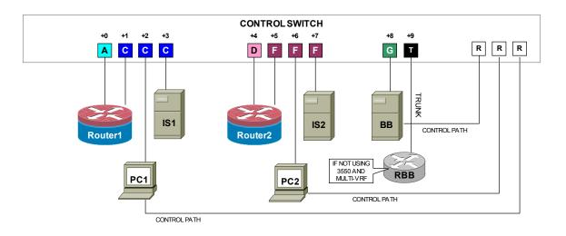
POD\_5 is using ports 1 to 10 on control switch 3. Therefore, the "T" port is FastEthernet0/10.
