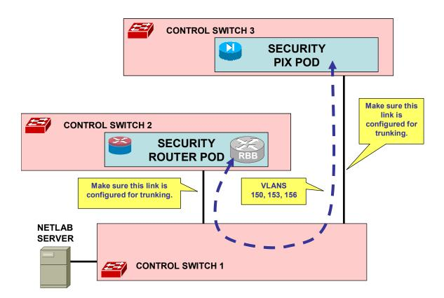
Next, we configure the physical RBB router. Begin by creating a virtual routing and forwarding instance for POD\_5 and POD\_6. Each VRF will represent a virtual RBB router. Each VRF requires a unique route descriptor in the form *rd:rd*. We will use the pod ID for the *rd* values.
