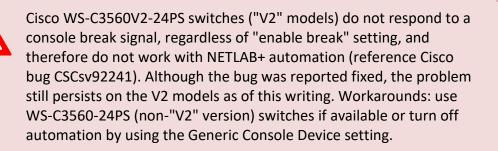
Please Note By default, these switches will not respond to a console break signal the same way routers do. There are two *environment variables* that affect this: **Enable Break** and **BOOT path-list**.
