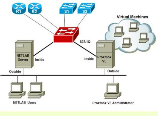
It is important that control switches are equipped with the minimum required image. For a supported list of device images for the control switch, please visit: https://www.netdevgroup.com/support/netlabve\_control\_devices.html#control\_switch
