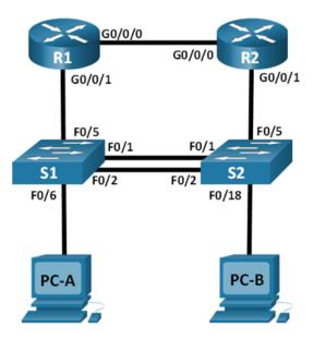
The *Multi-Device Pod (MDP)* features direct access to router and switch consoles. Integration with a separate *Proxmox VE* server supports up to 2 virtual PCs. *NETLAB+* can provide remote access to the keyboard, video, and mouse of the *Proxmox VE* virtual machines in the pod.
