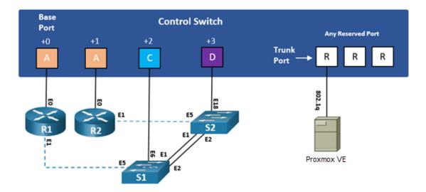
Ports are labeled **+0** to **+3** in the diagram and are relative to the *base port*. These ports must be consecutive on the same control switch. As with all pods, you choose a base port for the pod during pod installation. A control switch can support multiple pods. To determine the actual port numbers used for this pod, add the base port number to the relative port numbers shown in the diagram. For example, if the base port is 4, the actual port numbers will be 4 to 7.
