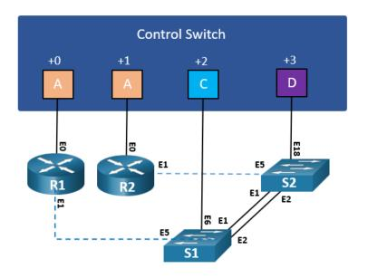
Then proceed to cable the access server lines as well as the PDU outlets; use *Section 3* from this guide as a reference.
