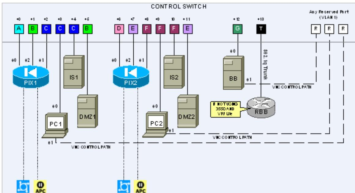
In the Security PIX Pod, RBB performs routing between network **A**, **D**, and **G**.
