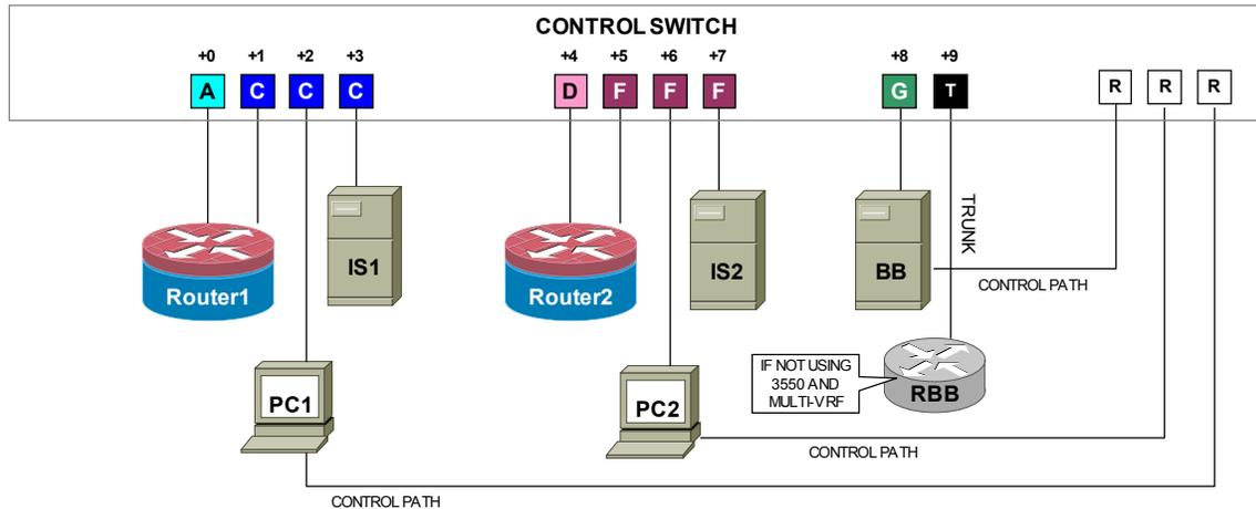
POD\_5 is using ports 1 to 10 on control switch 3. Therefore, the “T” port is FastEthernet0/10.
