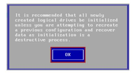
8. Use your arrow keys to highlight **VD-DAS1**. Press **F2** and select **Initialization > Start Init.** Select **Yes** to confirm Initialization of the HDDs. This process can take several hours.
