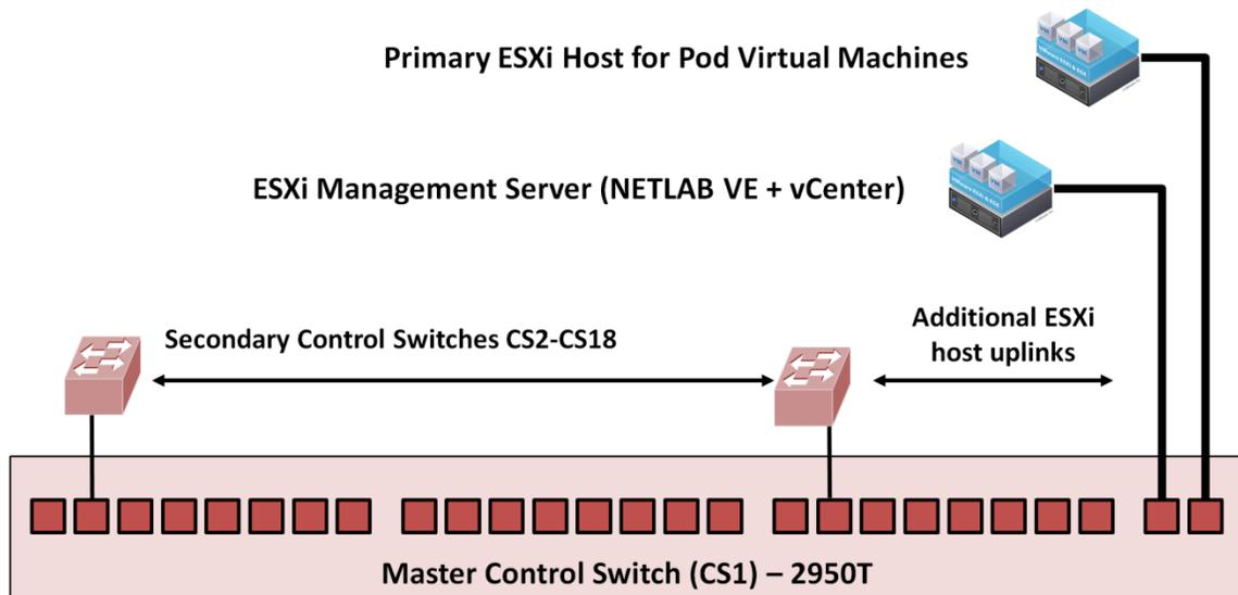
Best practice is to locate the master control switch in the same rack as virtual machine servers.
