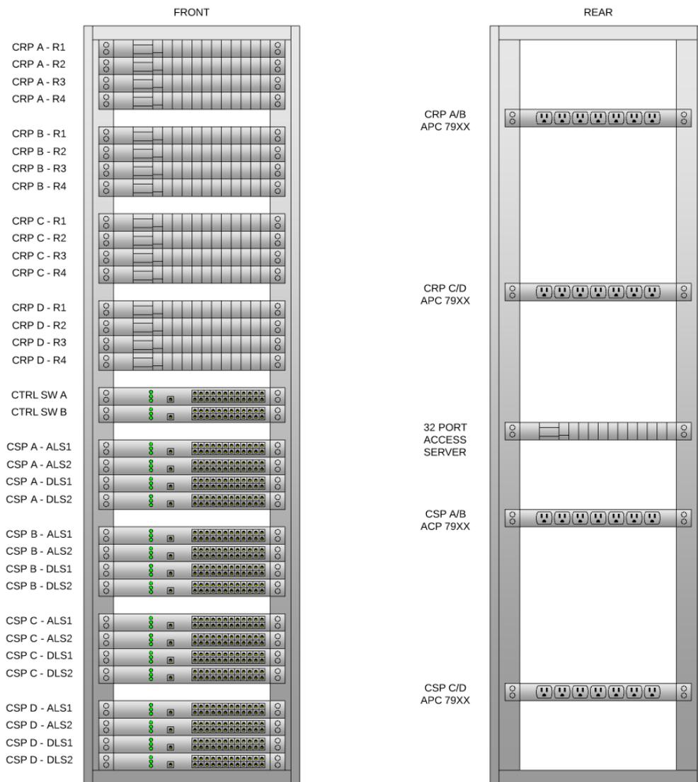
If space for power strip needed at bottom, coalesce open slots as needed.
